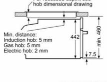
measurements in mm
